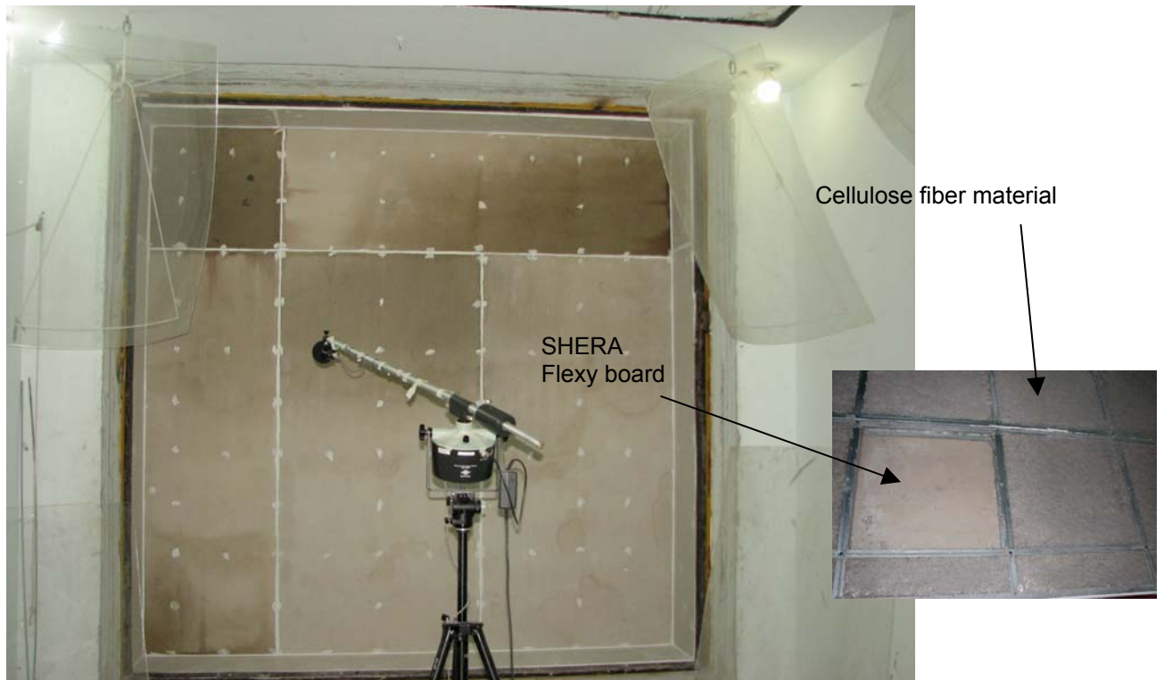
Figure 3 : Test set up of sample in the receiving room
