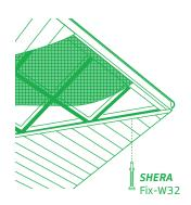
**3** Fasten *SHERA* Strip to steel studs with screw at at the middle from long-side edges.
